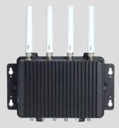
**Product Reference 1, Figure 1.** The eBOX800-511-FL supports 7th generation Intel® Core i5 or Celeron processors in an extremely rugged package that makes it ideally suited for deployment in edge traffic management and control systems (Source: **Axiomtek**)
